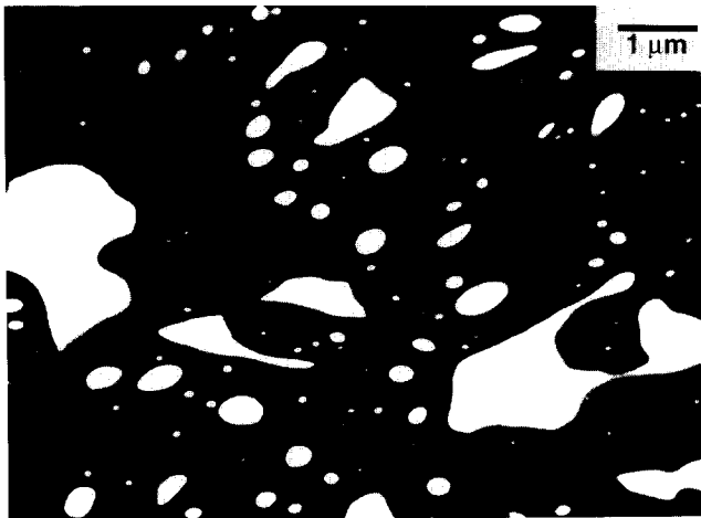
Figure 16 TEM photomicrograph of nylon 6/SAN 25/IA (75/17/8) blend taken from location 4 of the clamshell extruder operating at 200 rpm and extruder configuration A. Large irregular (2–4 μm) shaped particles are observed to co-exist with much smaller ones (~0.15 μm). The average particle size for this blend, \bar{d}_w = 0.55 \mu\text{m}
